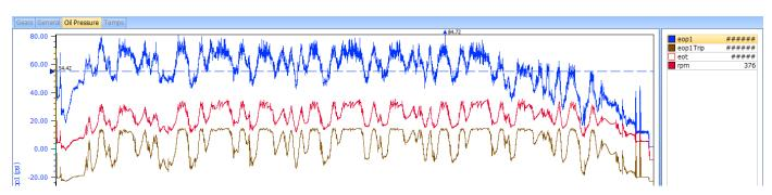
Below is an example of a noisy sensor, the bottom line is what the trace should look like and the top trace contains excessive noise.
