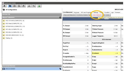
3. Ensure the steering wheel is straight then click "Autocalibrate All". After this process check that the steering angle is equal to the actual steering wheel angle at 90deg.
