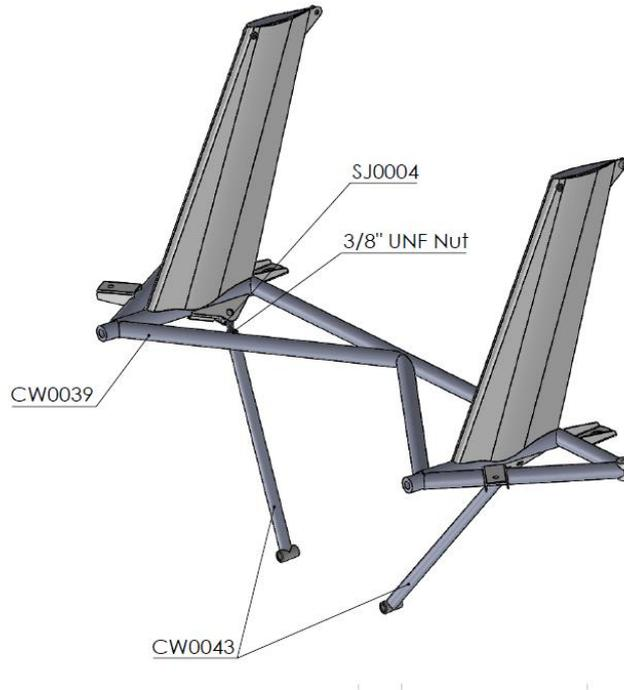
Figure 1 – SR8 Tail Frame Assembly
